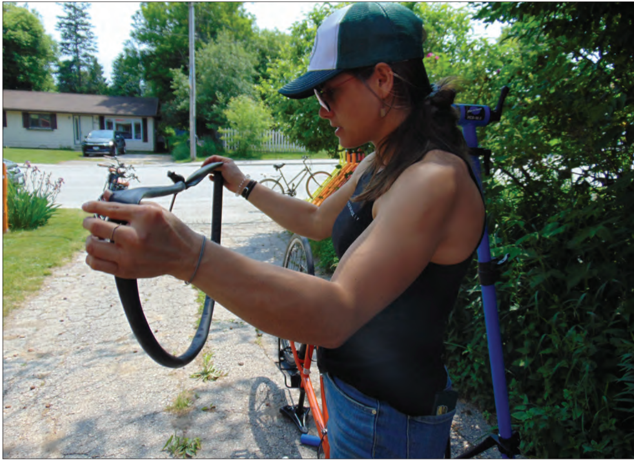
No extra tube? No problem! Tie a knot in the one you have.
