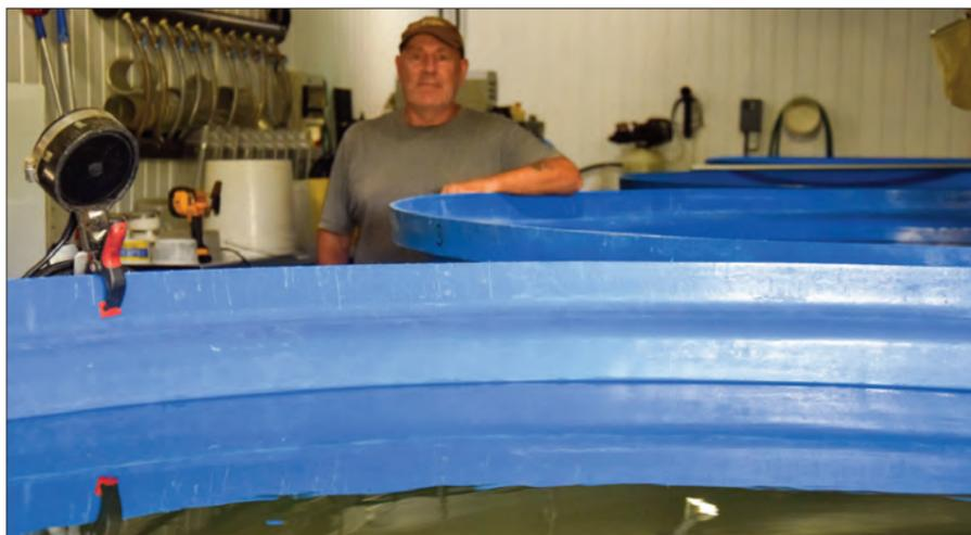
Renaissance man John Caselton stands behind one of a number of large tanks of his own design. The tanks use a solid knowledge of hydrodynamics to filter out solids and send them on to a biofiltering process that returns clean water in the closed system operation.
