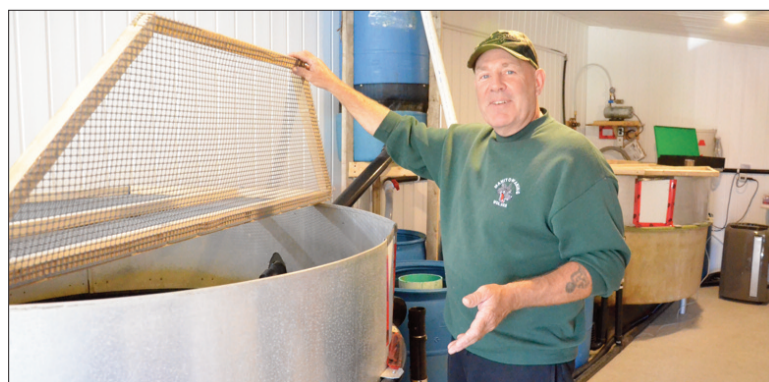
John Caselton of Caselton Aquaculture lifts the lid of one of the large stainless steel tanks he has been utilizing for his research into the best balance of temperatures, water movement and pH for raising various species of fingerlings.
