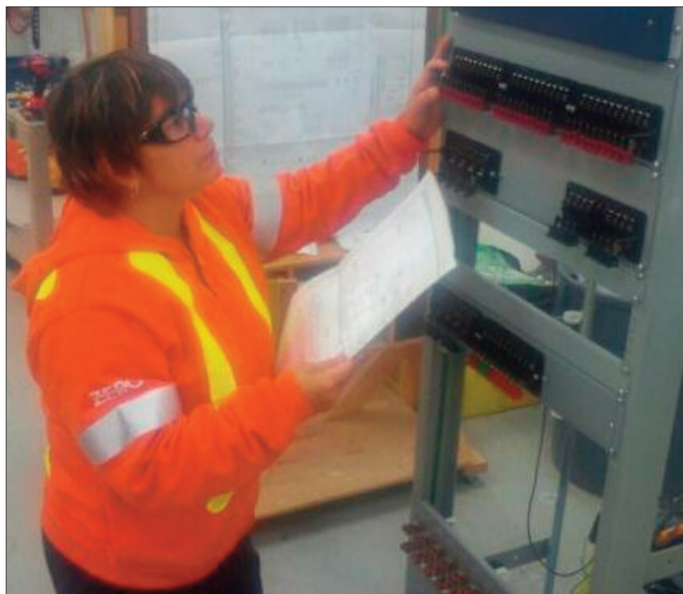
Construction and maintenance electrician Gina Simon assembles a rack to be used for a line protection system.
