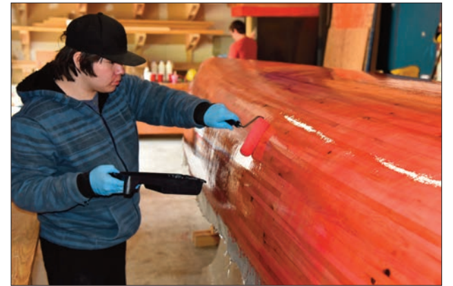
No details have been spared in the construction of this canoe. After sanding the body smooth, protective sealing coats have been applied to ensure it stays in optimal condition after facing the challenging waters of Lake Huron.
