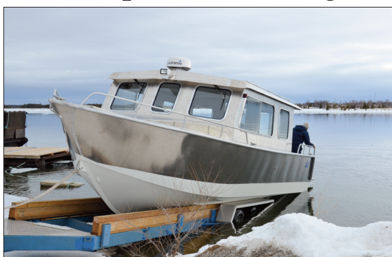
Henley Boat's custom designed 36-foot 14-man crewboat took its maiden voyage in the frigid, but mostly ice free, waters of the North Channel this past weekend powered by the 600-hp of twin 300-hp Yamaha outboard motors.
