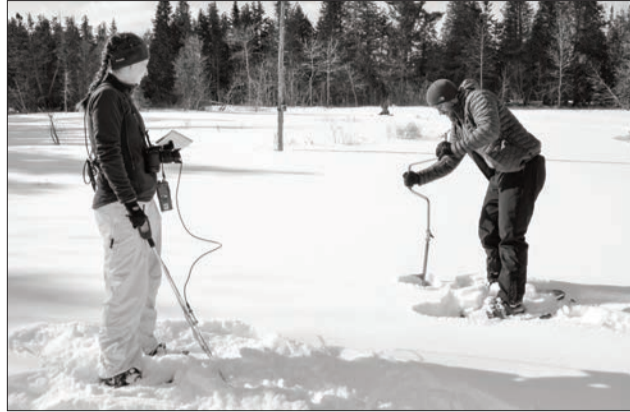
Joe Bienentreu augers a hole in the ice near a hibernating turtle allowing Donnell Gasbarrini to use a dissolved oxygen meter to record the oxygen level of the water.
