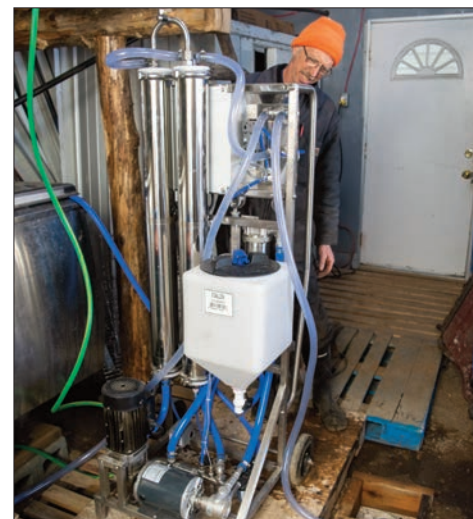
The newer reverse osmosis machine is not yet a well-accepted tool in the maple syrup world.
