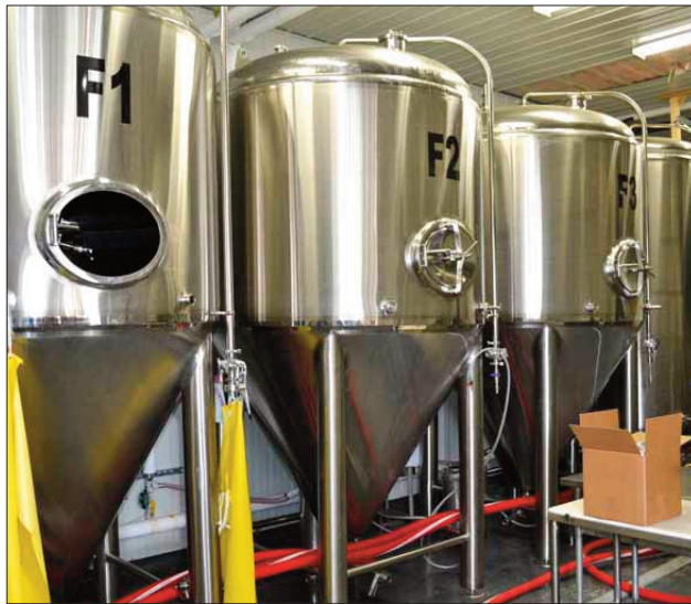
Large fermenting tanks hold 4,00 litres each, giving the brewery the ability to brew 220,000 litres of beer per month.
