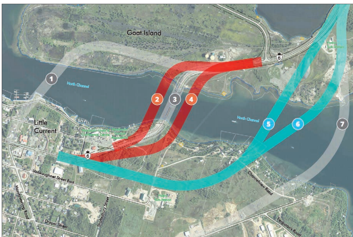
Possible entry and exit routes for each of the bridge options. Colour on the graphic matches the swatches with the individual descriptions above. Note that the first and seventh option, in grey, are no longer being considered for the project. The third option, also in grey, shows the current alignment of Highway 6 as it crosses the swing bridge.
