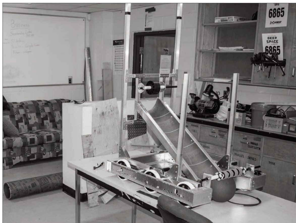
This year's build is a complex system of a riveted frame, mechanized rollers and a six-wheel drive system. It uses the concrete forming tube, arranged within a metal track, to shoot balls while completing missions. At the time of the FIRST president's visit, the team was exploring its options for side bumpers.
