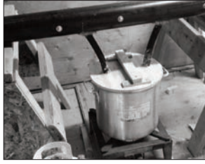
Students created a steamer from PVC pipe with a rack in the middle to steam all six sides of the 2/6 inch white ash strip.
