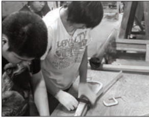
After steaming the wood, students bend it to form a lacrosse stick.
