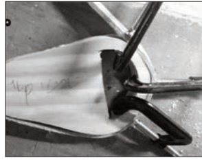
Clamps are used to hold the wood strips together as they dry.
