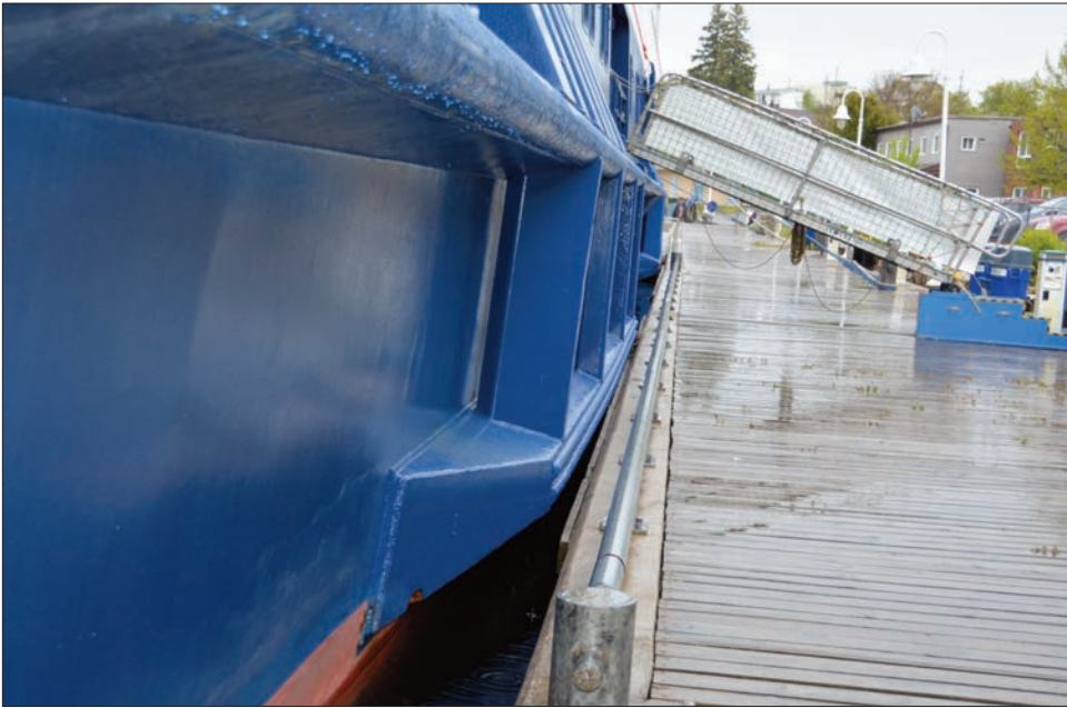
The Victory I's bumpers caused some damage to the Little Current downtown wall last month, the result of high water levels and the boat's construction. Measures to protect the dock mean the cruise ship can once again dock downtown.
