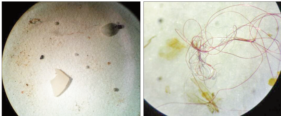
The greatly-enlarged photograph on the left is an example of a microplastic element found in a Lake Erie fish, while the photo on the right shows microfibres that have made their way into the lakes, our water supply, and the stomach of a fish.
