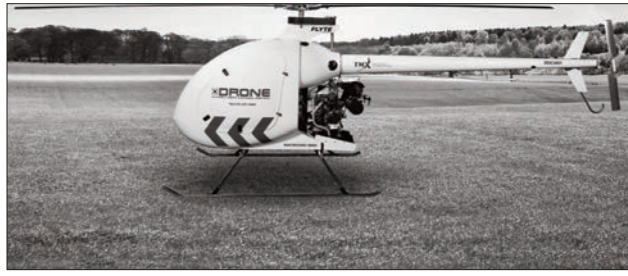
The Condor, a larger drone model that is gas-powered and can transport 400 pounds of cargo up to 200 kilometres per tank at 120 kilometres per hour. It is best suited for extremely remote locations such as fly-in reserves.
