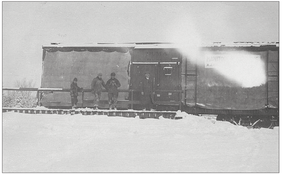
Specialized open-sided turkey boxcars were built by A.J. Wagg to bring his turkeys safely to market. The cars provided ventilation in the summer months, but special curtains protected the delicate birds from the ravages of winter.
