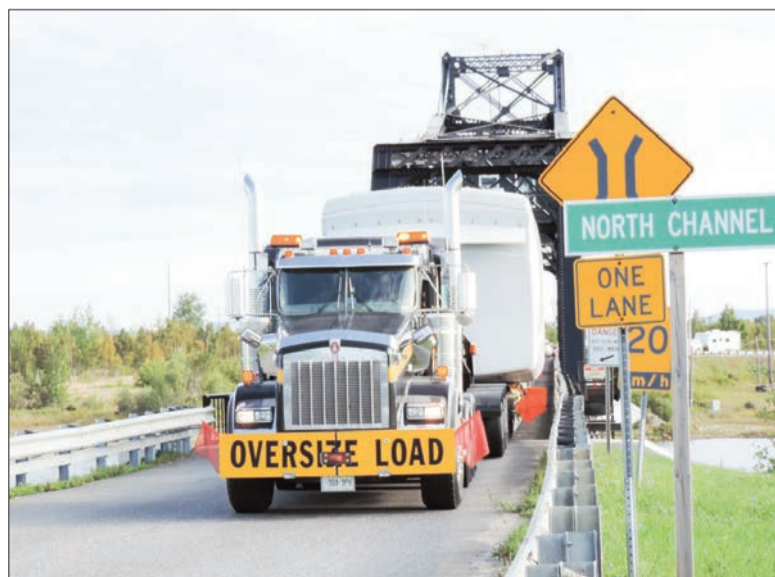
A turbine nacelle crosses the bridge on Monday morning. The nacelle houses all the generating components including the generator, gearbox, drive train and brake assembly.
