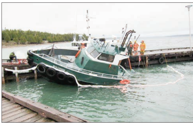
The tug Wyn Cooper sunk in South Baymouth earlier this month after waves swept over the boat and into an open hatch. The Tehkummah volunteer fire department is seen above pumping the vessel out.
